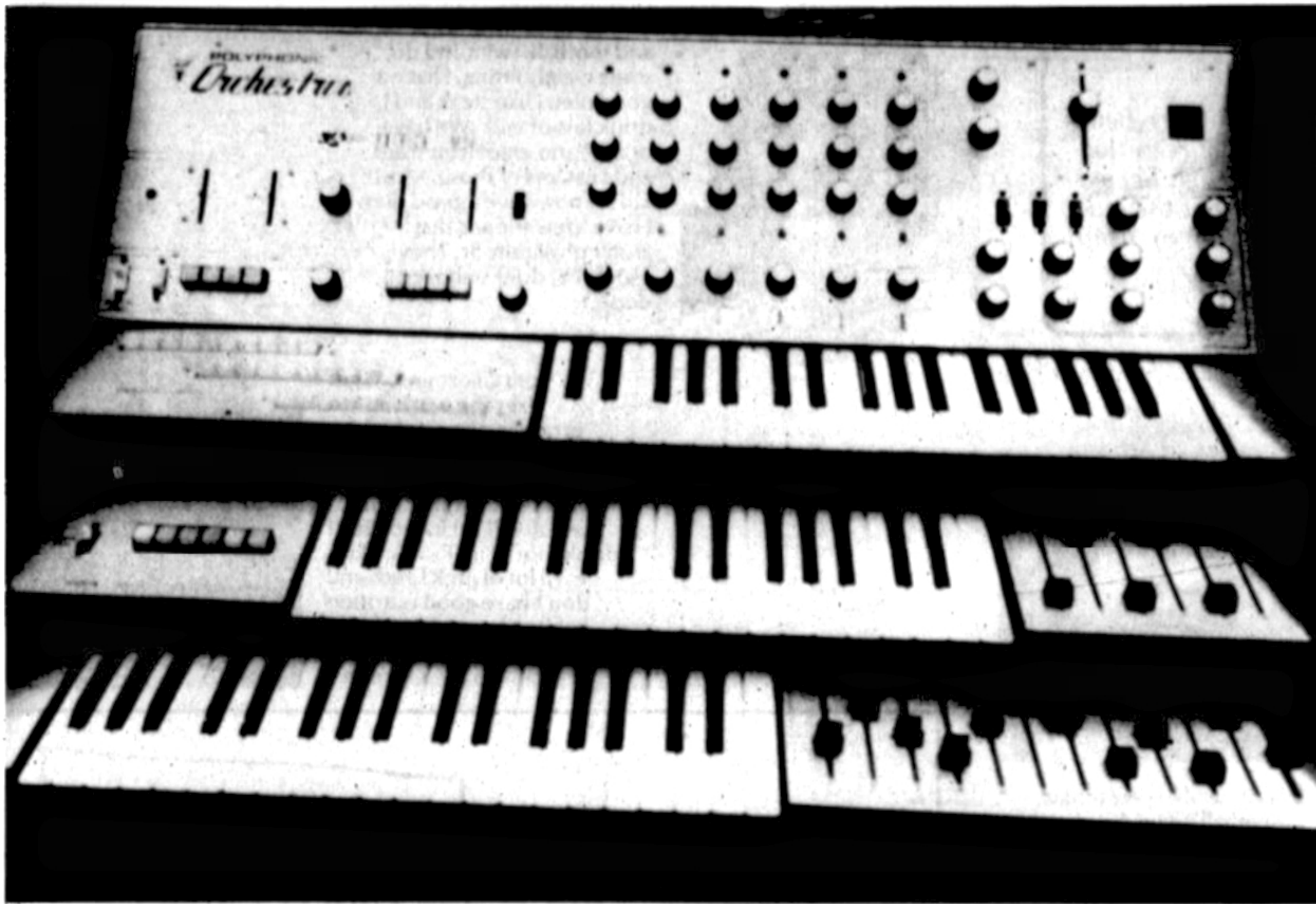
The Orchestron's top keyboard controls synthesizer sounds; its lower two play not only notes but entire chords, which synthesizers cannot do, of up to 12 instruments at a time.
